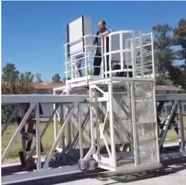
Figure 16. Pipe Conveyor with Rectangular Frame and Compact Maintenance Trolley
