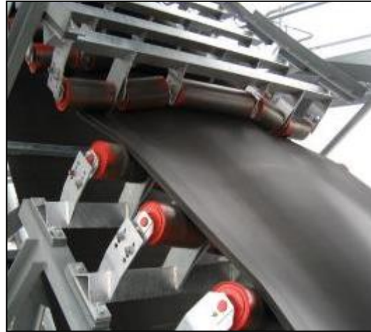
Figure 17 – left side: Original inflection zone with standard vari-troughing idlers.
