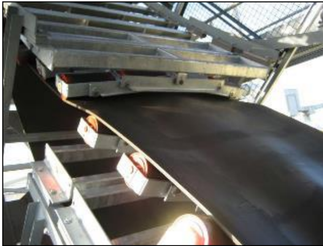
Figure 19 – left side: FEI's (Fully Equalised Idlers) at the inflection zone.
