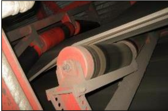
Figure 17 – left side: Original inflection zone with standard vari-troughing idlers.
