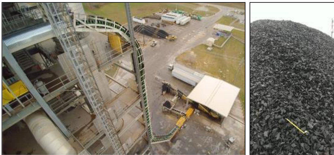
Figure 5 – Left: Background shows shredder system and storage pile. Right: Close-up of tyre shreds in storage pile.
