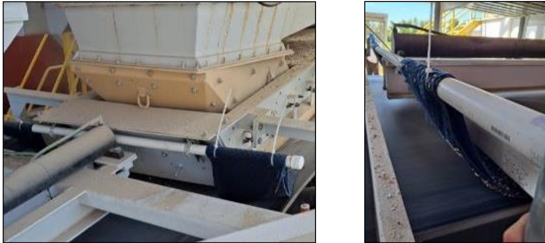
Figure 21 – Edge Brushes; at bottom belt (left) and at top belt (right)
