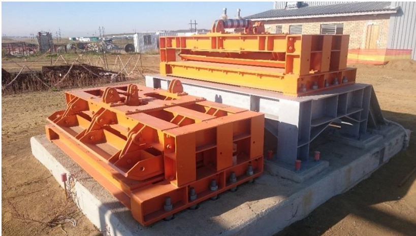
Figure 9 - Let down belt clamp for lowering the belting down the shaft
