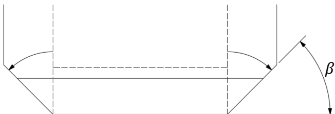
Figure 4. Transfer chute cross-section variation for a constant width centre section. Flow depth reduces.
