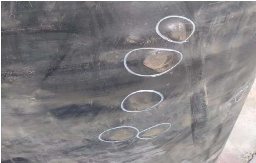
Figure 8, Project example 2, cord end depressions in splice are indicative of cord movement
