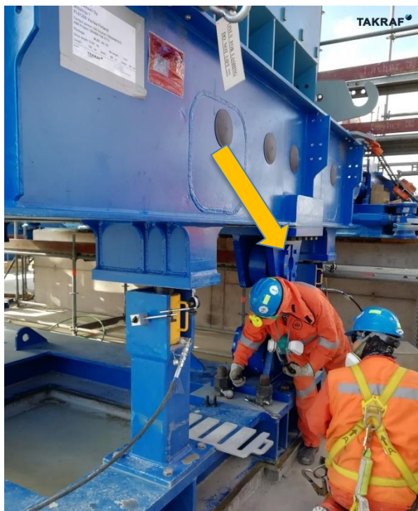
Figure 9: Motor alignment during assembly.
