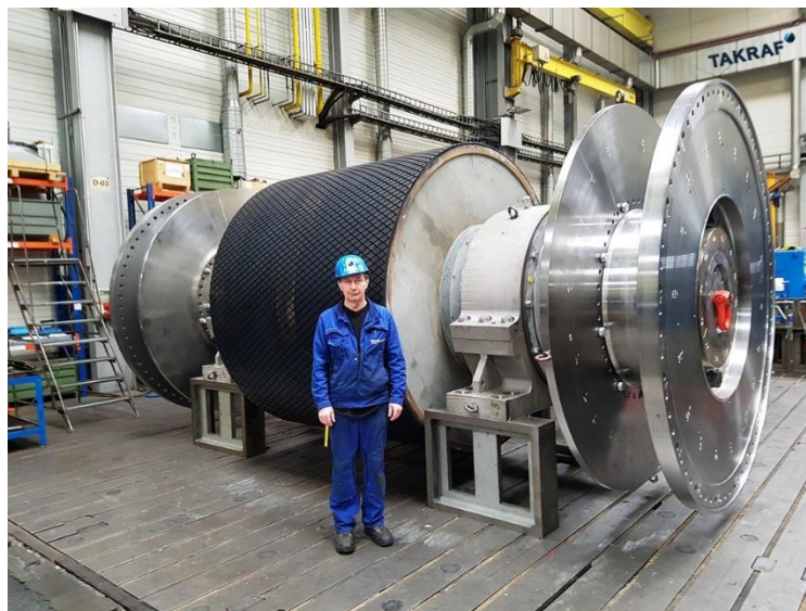
Figure 11: Drive pulley with brake disk and membrane coupling half at the fabrication facility in Lauchhammer, Germany.
