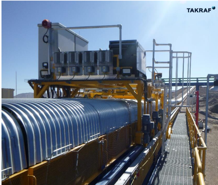
Figure 20: Maintenance cart for safely lifting the belt and replacing the idlers.
