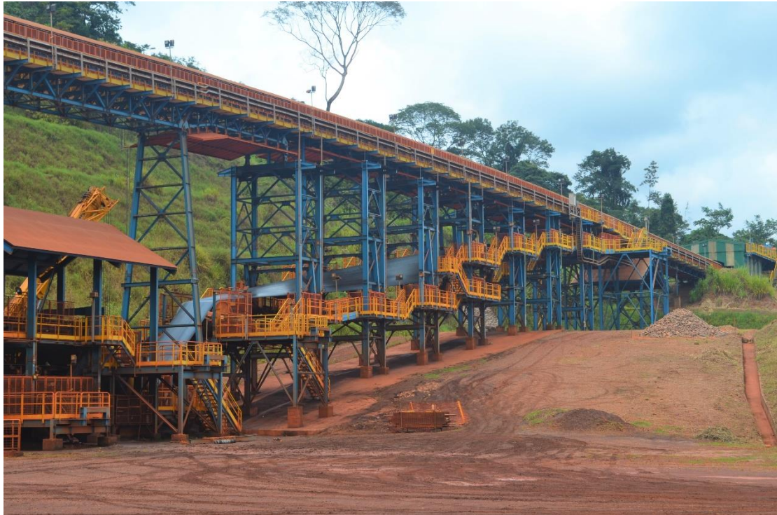
Figure 18. World's longest belt turnover of 72 m for an ST-8000 N/mm belt rating.
