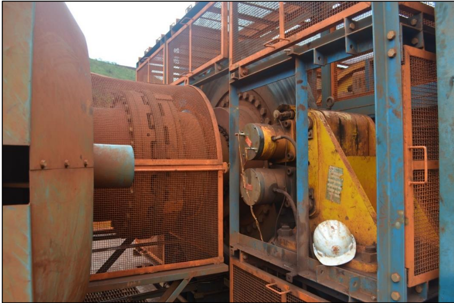
Figure 15. One of seven low speed brakes with both digital and proportional types.
