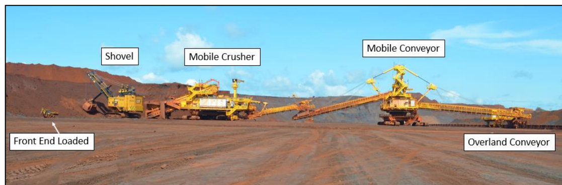
Figure 9. Truckless mining. Material is directly loaded onto the conveyor system.
