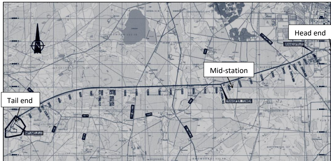
Figure 1: Impumelelo overland conveyor route
