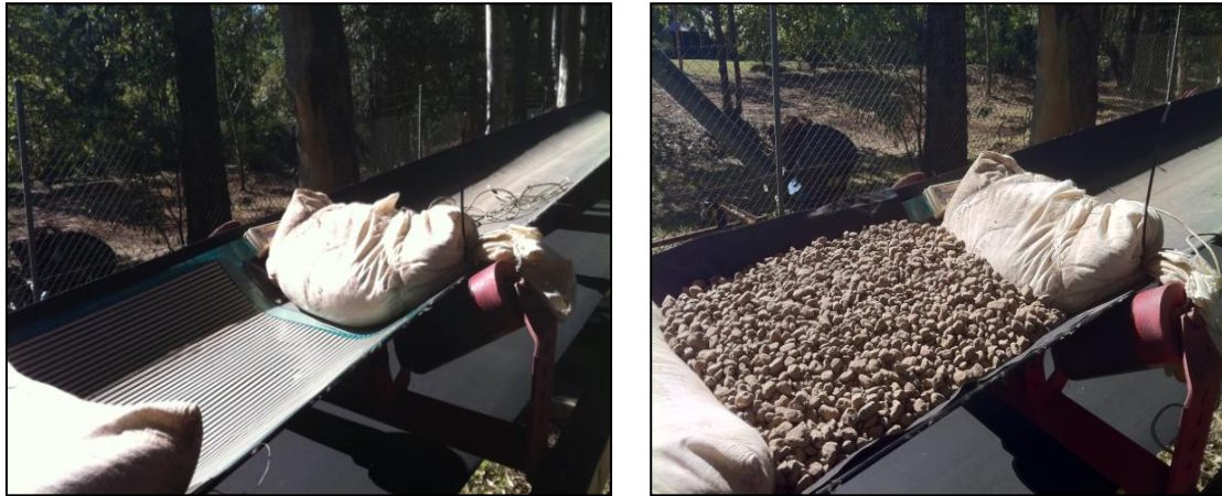
Figure 7. Experimental set-up to measure belt surface pressure during transportation
