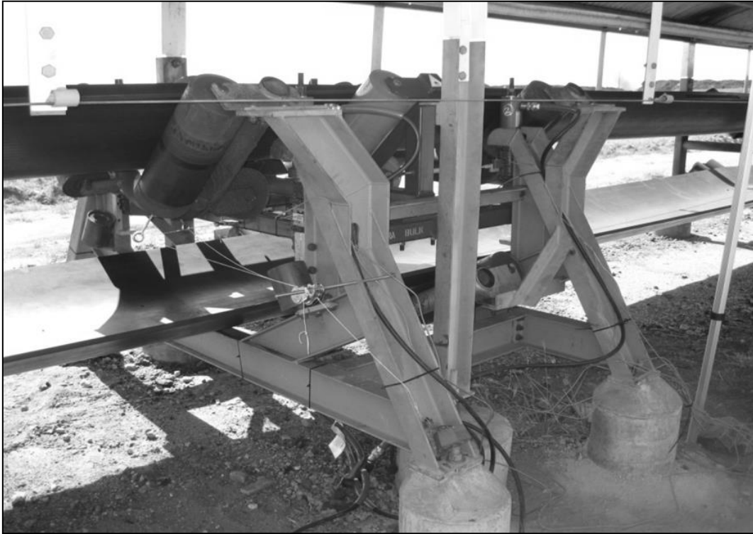
Figure 20. Main resistance measurement apparatus pictured during field tests
