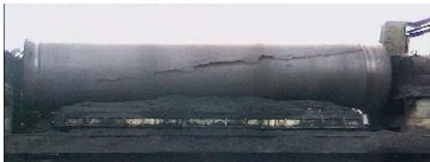
Figure 1: An example of a single video frame showing a conveyor belt splice which exhibits some delamination.
